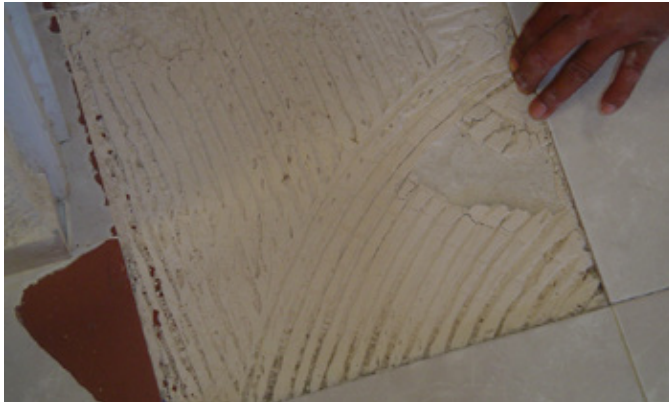
Thinset bond defective install. Photos courtesy of Dave Gobis.
