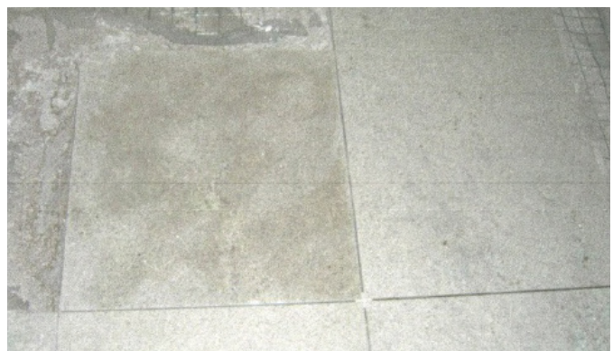
Photo 5: Mock-up test showing sealed stones vs. an untreated piece
