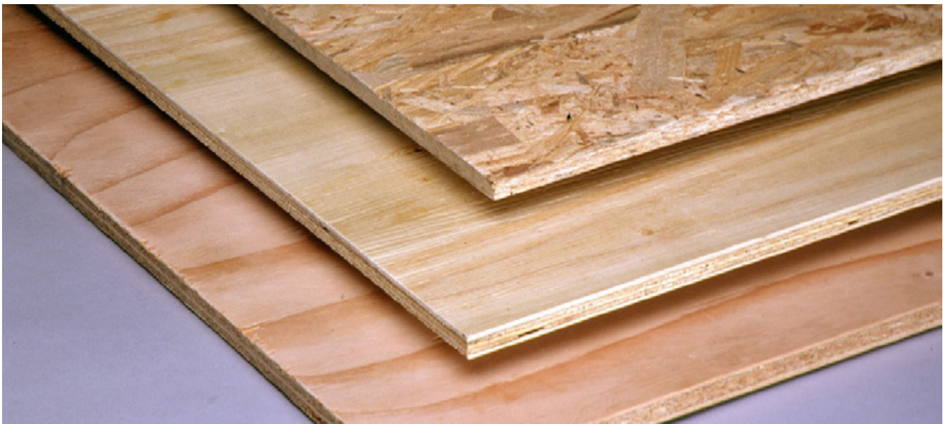
The traditional and proven wood subfloor thickness for tile installations on joists spaced 16 in. (406 mm) is two layers of 5/8 in. or 19/32 in. (15.5 mm) thick plywood.
